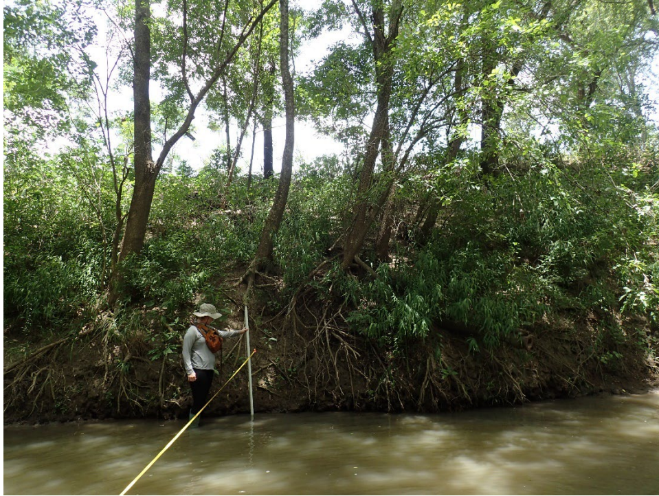
Figure 4-13: SARA intern conducting habitat transect at station 12802. Note bank failure, exposed soil and tree roots.
