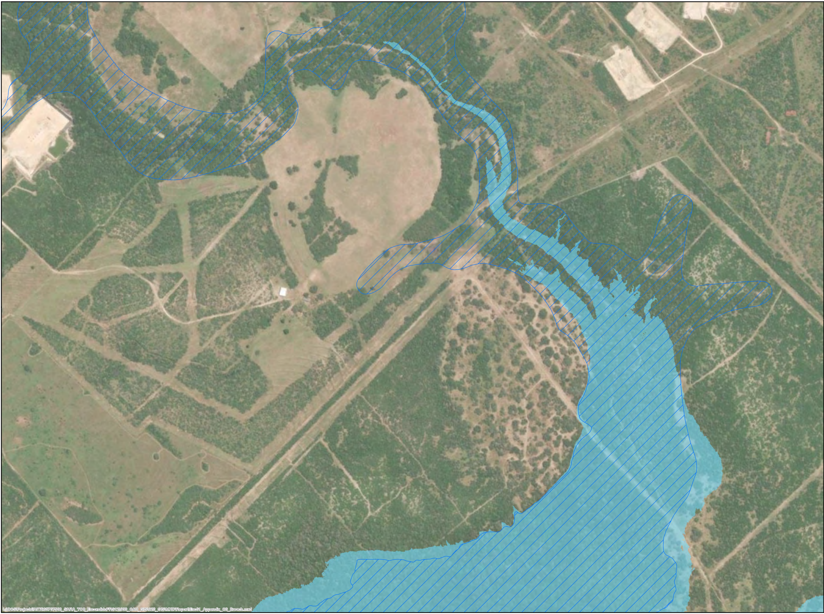
Escondido Creek Watershed FRS No. 1 Karnes County, Texas Figure C-6 FRS No. 1 and FRS No. 13 FBH Breach Inundation Map 11 of 13
