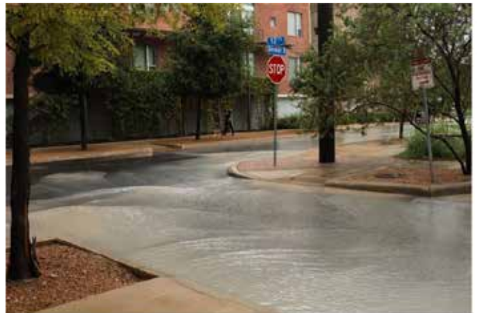
Sediment from a construction site running off into the street, where it will be carried to a storm drain and then directly into a river.
