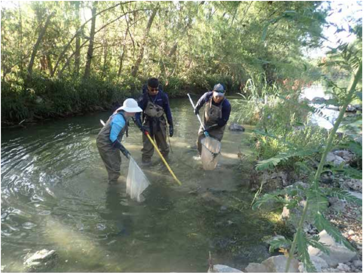
San Antonio River Authority staff conducting a biological sampling for fish with a backpack shocker on the San Antonio River at Camino Coahuilteca, just downstream of downtown San Antonio. The backpack shocker stuns the fish to allow capture, measurement and identification. Fish are revived and released back into the stream.
