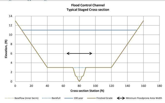
Figure 36: Typical Staged Cross-section for Flood Control Channel
