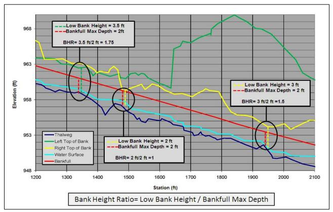
Figure 16: Method for Calculating Bank Height Ratio (BHR)
