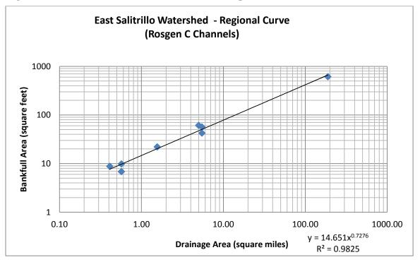
Figure L.4: Bankfull Cross-Sectional Area Comparison
