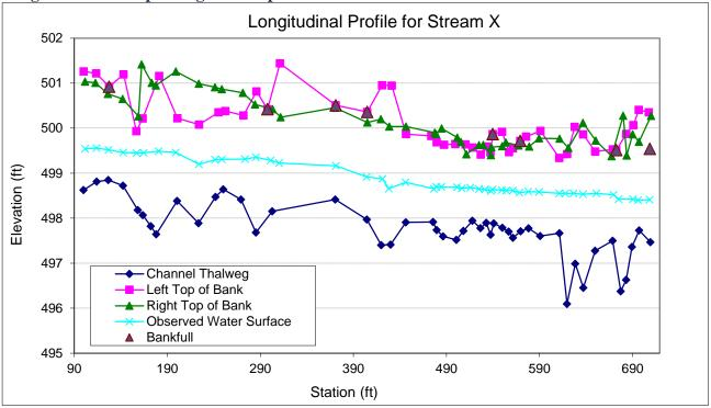
Profile measurements are used to develop ratios like those developed for reference reaches (see *Chapter 7*) to assess the degree of departure from reference conditions.
