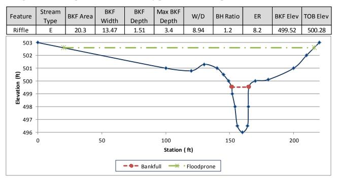
**Figure 10: Example cross-section survey plot and bankfull parameters**
