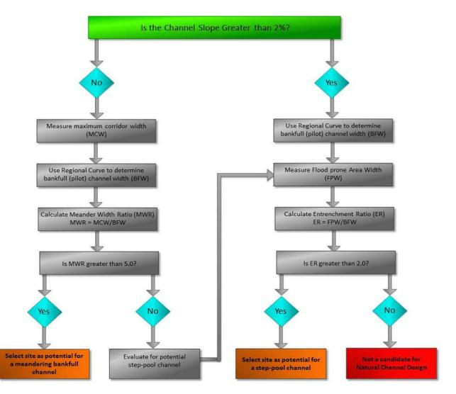
The first step is to look at the channel and valley slope. If the channel slope is less than 2%, a meandering pattern may be possible given that the meander width ratio (MWR) is greater than 5.0 following the steps on the left side of the flow chart. If the (MWR) is less than 5.0, a step-pool design may still be feasible if the Entrenchment Ratio (ER) is greater than 2.0 (following the step on the right
