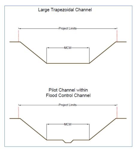
Figure 1 – Maximum Corridor Width Measurement
