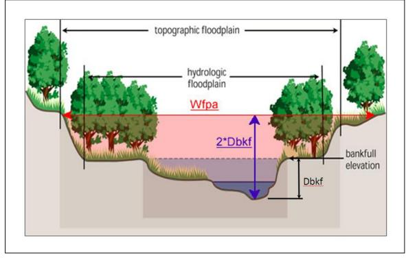
Figure 17: Method for Calculating Entrenchment Ratio
