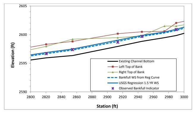
**Figure 13: Comparison to Observed Bankfull Indicators with HEC-RAS Water Surface Profile Simulations**
