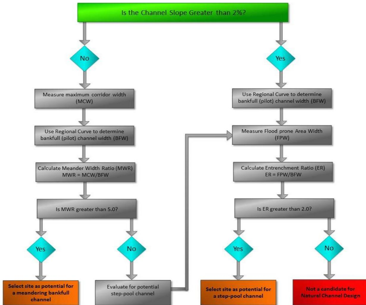
The first step is to look at the channel and valley slope. If the channel slope is less than 2%, a meandering pattern may be possible given that the meander width ratio (MWR) is greater than 5.0 following the steps on the left side of the flow chart. If the (MWR) is less than 5.0, a step-pool design may still be feasible if the Entrenchment Ratio (ER) is greater than 2.0 (following the step on the right
