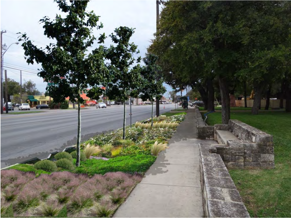
Rendering showing how roadside bioretention can be retrofit into the right-of-way to intercept street runoff through curb cuts, Broadway Street, Witte Museum, San Antonio, Texas. Source: Bender Wells Clark Design
