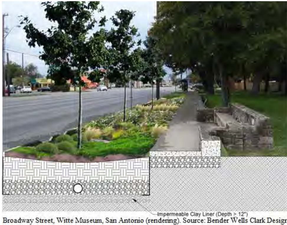
Figure B-13-20. Bioretention area with clay liner and lateral hydraulic restriction barriers
