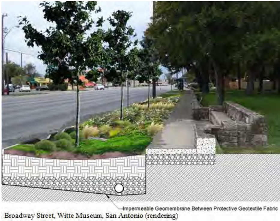
Figure B-13-21. Bioretention area with geomembrane layer
