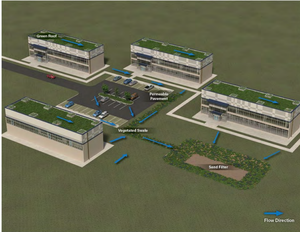
Figure B-12-3. Example of commercial treatment train
