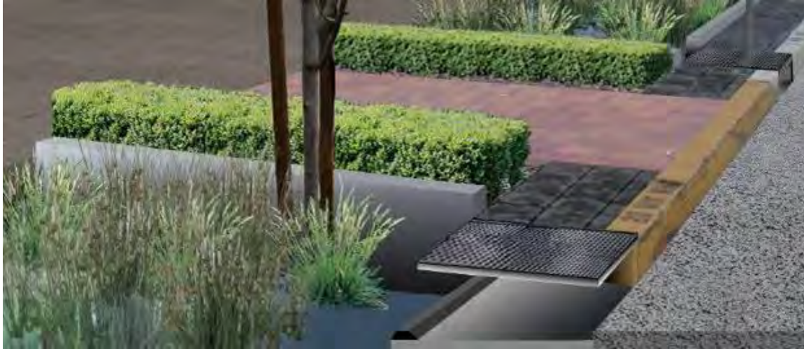
Figure B-13-6. Rendering showing a covered curb cut with a sump. Source: City of San Diego LID design Manual
