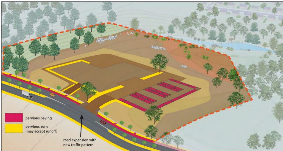
Figure 1-14. Site example demonstrating placement of pervious material (red) and opportunities to minimize connected impervious area (yellow)
