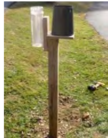
Figure 4-22. Manual (left) and tipping bucket (right) rain gauges. Source: Tetra Tech
