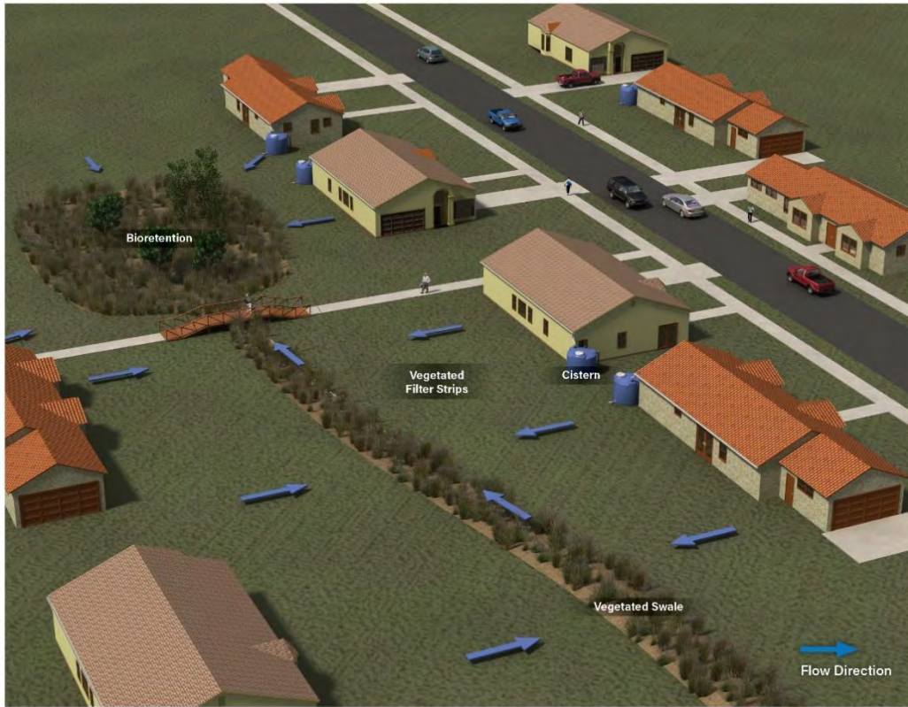
Figure B-12-2. Example of residential treatment train
