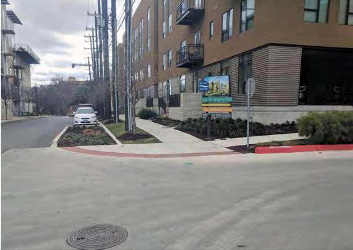
Figure 1-16. Intersection pop-out, River House, San Antonio, Texas.
