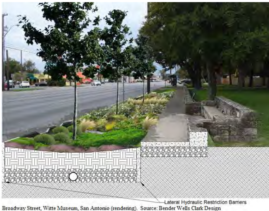
Figure B-13-19. Lateral hydraulic restriction layers in a roadside bioretention area prevent horizontal seepage while allowing infiltration at a safe depth
