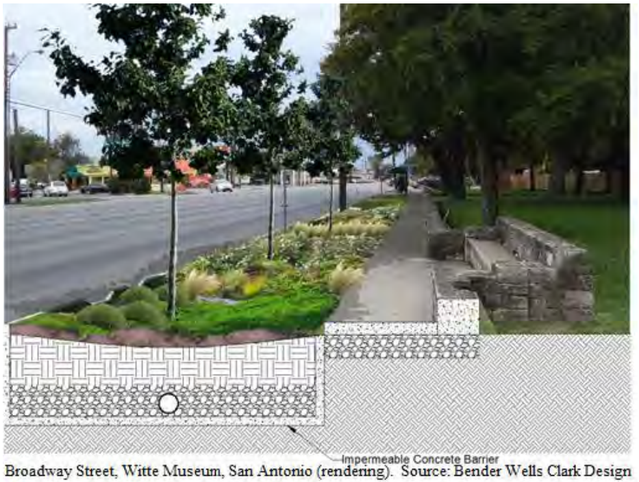
Figure B-13-22. Bioretention area completely lined with concrete barrier (planter box)
