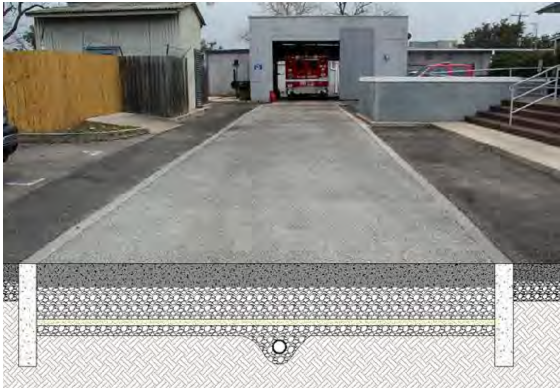
Figure B-3-11. Permeable pavement showing example cross section with trenched underdrain at Alamo Heights Fire Station, Alamo Heights, Texas. Source: Tetra Tech
