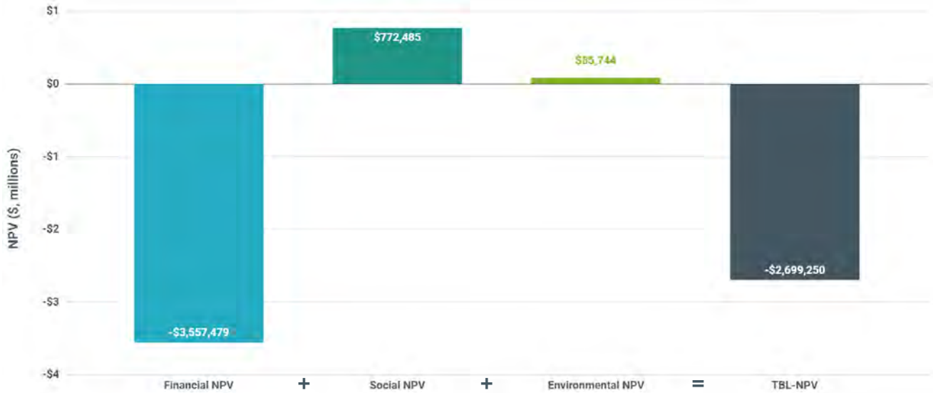
Figure 1. Comparison of the Expected TBL-NPV of Financial, Social, and Environmental Results For Site 8 (Subbasin 560) | Net Present Value Over 50 Years Discounted at 3%
