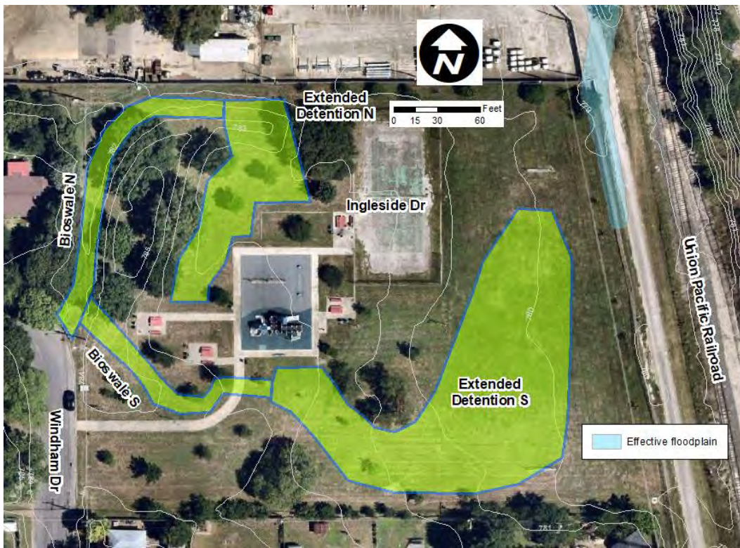
Exhibit E-3 Proposed BMPs on Subbasin 70 Site
