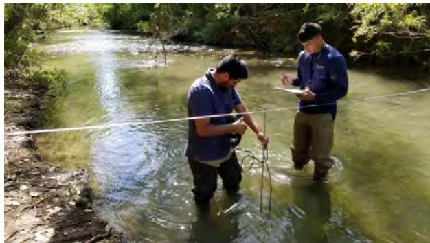
Figure 63: River Authority staff collecting ambient flow measurement the day before a stormwater event.
